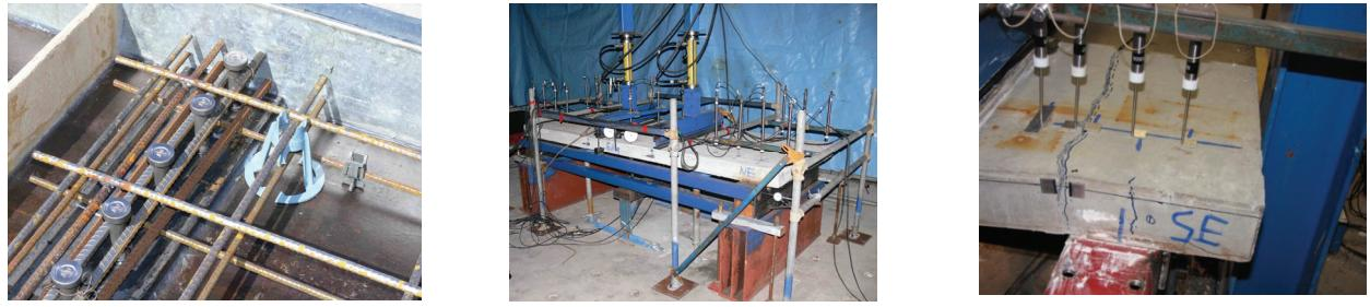
(a) Studs welded to steel base plate protrude through two layers of mesh & other bars      (b) Test set-up (used prior to constructing universal test rig)      (c) Fracture of top mesh bars confirmed the bars were fully anchored past inner edge
